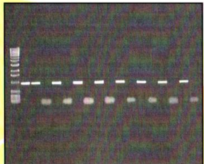
Fig. 2: Laboratory equipment contaminated with plasmid DNA was cleaned with LTK-008. Potential DNA residue was amplified in a polymerase chain reaction* (800 basepair plasmid-specific band) and deposited on a gel. Length standard (lane 1), 800 bp amplified product (lane 2). Lanes 3-18: tests of the various surfaces before and after cleaning with LTK-008. Stainless steel (lanes 3+4), aluminium (lanes 5+6), polypropylene (lanes 7+8), polystyrene (lanes 9+10), polyethylene (lanes 11+12), glass (lanes 13+14), pipetter (lanes 15-16), work surface (lanes 17+18).
