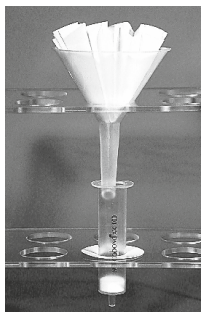
Figure 1 Correct use of the NucleoBond® Filter, NucleoBond® Column placed in a Plastic Washer
