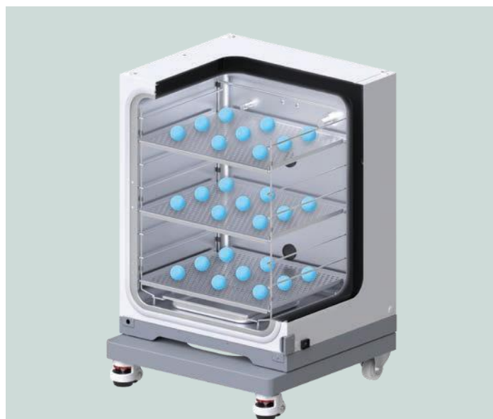
Position of the 27 sensors to verify equal temperatures at different locations.
